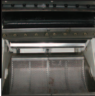
Tangential feed cutting chamber allowing for better ingestion of feedstock
