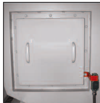
Side cleanout door with safety interlock
