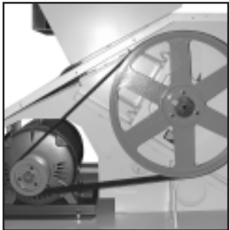
Dual sheaves offer additional cutting inertia
